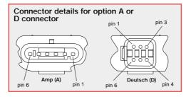
When connecting the sensor, care should be taken with the correct connections. The sensor is provided with indefinite reverse polarity protection and short circuit protection between output to GND (Black), but if the outputs are connected to the supply
